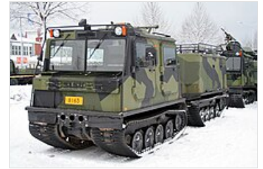
Sisu Nasu NA-110 tracked transport vehicle of the Finnish Army. Most conscripts receive training for warfare in winter, and transport vehicles such as this give mobility in heavy snow.
